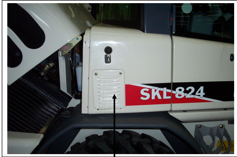
Air intake panel back in place.
